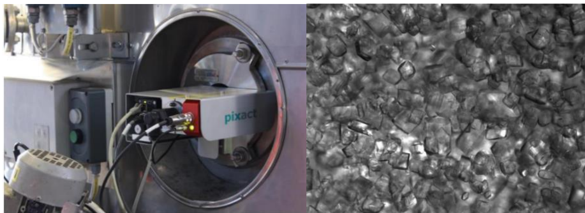
Figure 12. Installation on the boiling pan sight glass (left) and example image of the crystal suspension (Hannu et al. 2019).
